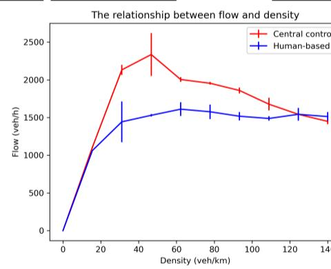
In the human-based model it is more common to have congestion at any section of the highway at the same time due to a lot of over-speeding and breaking
